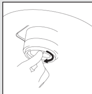
Remove the reverse-threaded impeller
